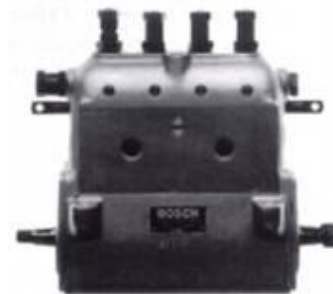
The first Diesel Injection Pump for cars, produced by Bosch in
