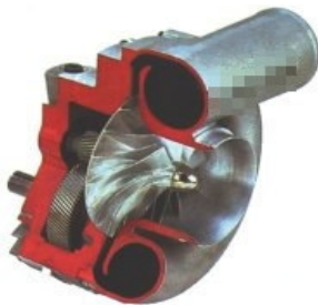
A mechanically-driven centrifugal supercharger. Note the speed-increasing gears in the case behind the impeller.
